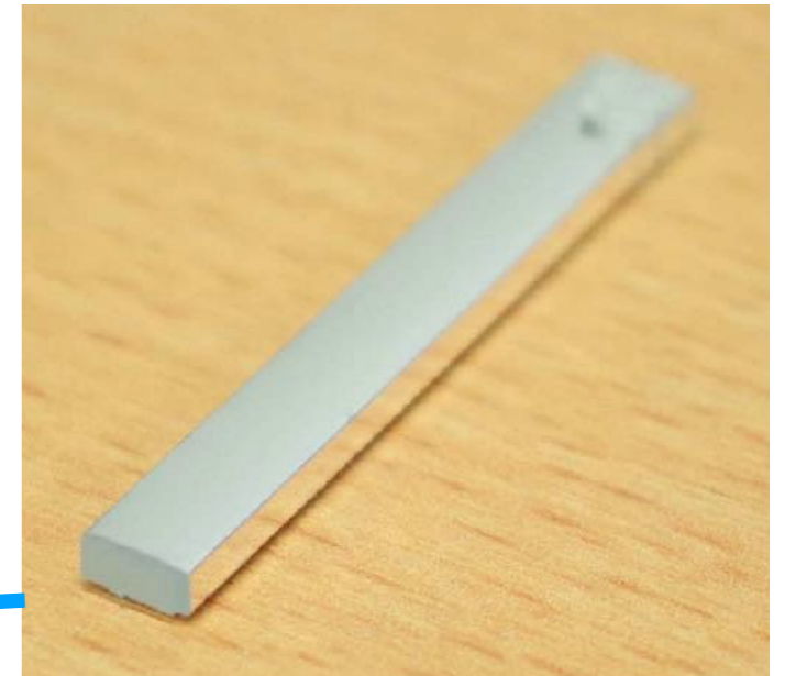
Scintillator (45 x 5 x 2 mm 2 )
