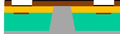
16. Removing DLC on the Cu plating
