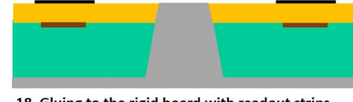
18. Gluing to the rigid board with readout strips
