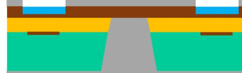
14. Etching for the resistive cathode pattern
