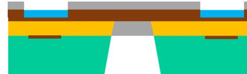
13. Connection to top anode & making anode strip
