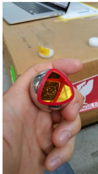
図 9.14 Spherical Mounted Retro-reflector(SMR)
