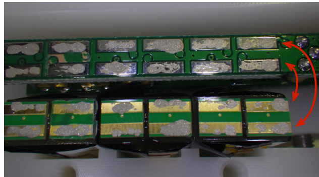
Figure 5.27: PCB (top) and SiPMs (bottom) after disassembling. The red arrows show the glued areas before disassembling.
