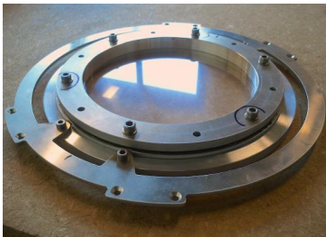
Figure 6.1: RDC mockup ( 230 \mu\text{m} thick Mylar foil).
