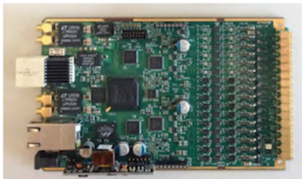
Figure 2.19: Pictures of the WaveDREAM. Left : Single board for 16 channels. Right : Crate for the boards.
