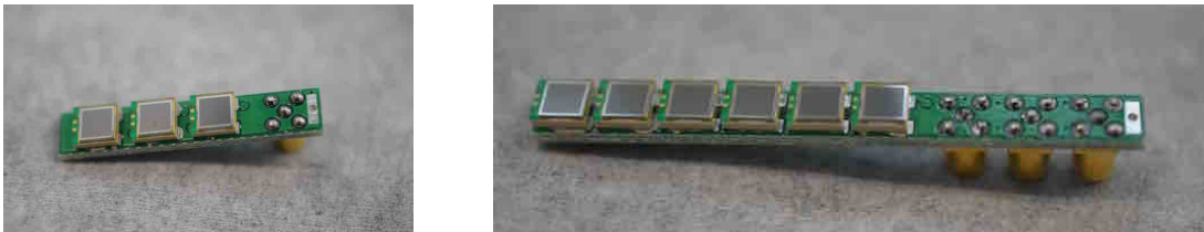
Figure 3.8: Left : PCB for a scintillator with a width of 2 cm. Right : PCB for three scintillators with a width of 1 cm.
