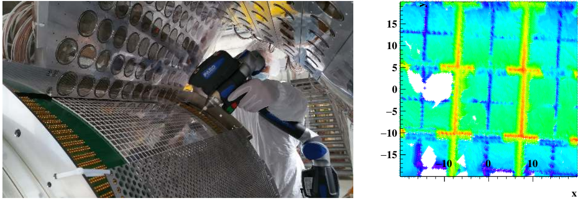
Figure 5.3: (Left) The surface of the MPPCs is scanned with the laser scanner [48]. (Right) An example of the measured height (perpendicular to the surface) distribution. The MPPC package structure (hosting four chips) is visible.
