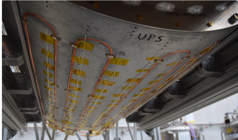
Fig. 2.42: The support structure viewed from the bottom side [7]. Cooling pipes and laser optical fibers can be seen.
