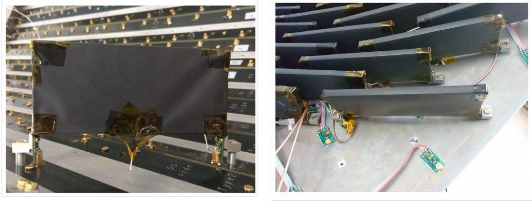
Fig. 2.38: (Left) A mounted flat-type counter on the backplane. (Right) Mounted L-shape counters on the inner step of the support structure [7].
