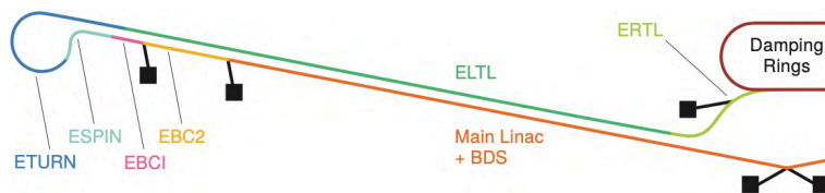
Figure2.5 Schematic of the main linac layout [19]
