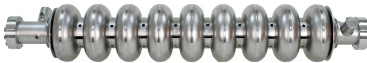
Figure2.6 A superconducting nine-cell 1.3 GHz resonator (cavity) [20]
