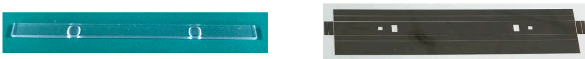
FigureA.9 Scintillator strip (left) and reflector film (right) for the double-side readout layer.
