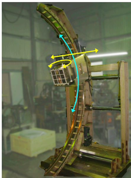
Figure 3.16 Mover for the reference counter. The arrows shows the degree of freedom [44].
