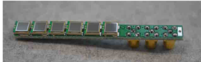
Figure 2.45 PCB for scintillators with a 2 cm width (left) and a 1 cm width (right).
