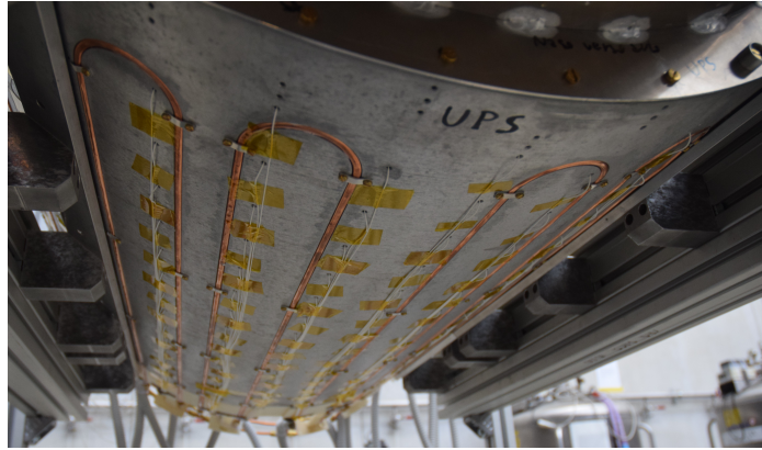
Figure 4.54: Backside of the support. Cooling piles and fibers fixed by tape are installed
