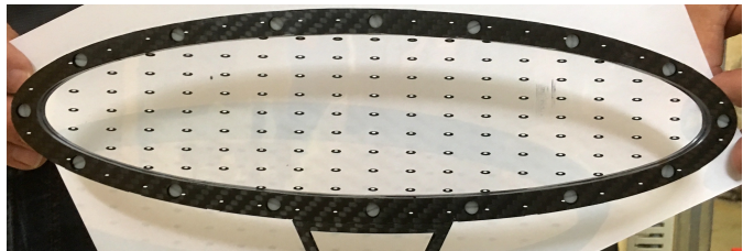
Figure 3.16: Target in MEG. There are six holes for vertex study and for monitoring target alignment.
