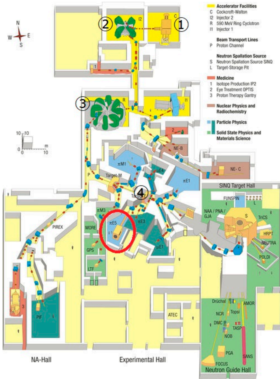
Figure 3.8: Overview of Beamlines in PSI. (1) Cockcroft-Walton injector. (2) Injector. (3) 590 MeV Ring Cyclotron. (4) Target E. \pi E5 area is encircled in red.
