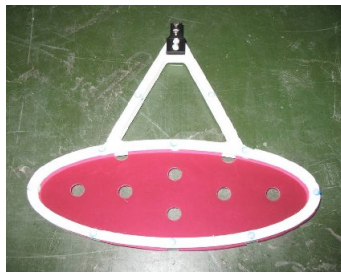
Figure 3.16: Target in MEG. There are six holes for vertex study and for monitoring target alignment.
