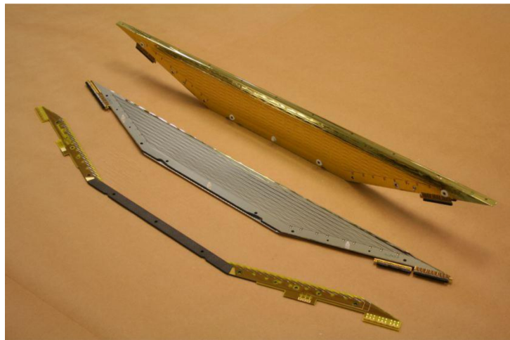
Figure 3.19: Element of a drift chamber module.
