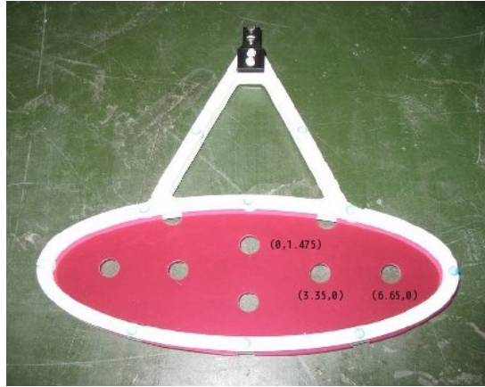
Figure 3.10: Muon stopping target.
