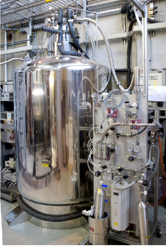
Figure 3.47: Liquid xenon tank and gaseous purification system.
