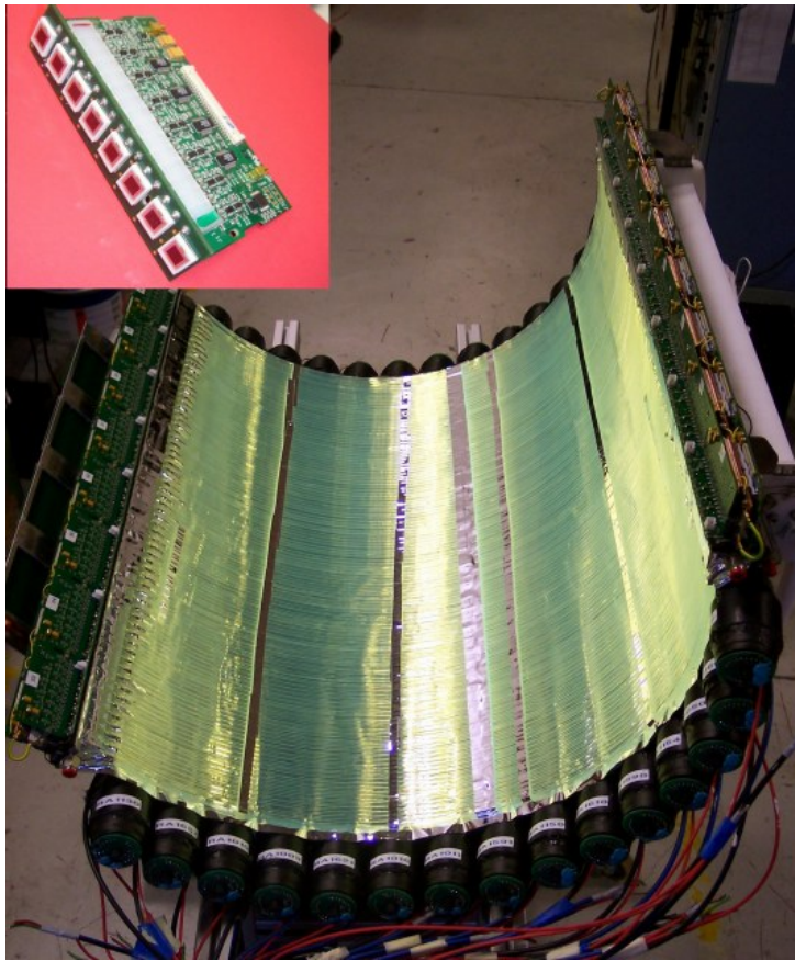
Figure 3.29: Timing z counter and 1\text{ cm} \times 1\text{ cm} APD for scintillation fibers. The fibers are mounted on timing \phi bars.
