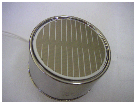
Figure 3.35: Photo-multiplier tube for the LXe detector. Aluminum stripe makes a flat response.
