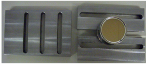
Figure 7.1: Lead collimator with 1.8 cm thickness in 2008 (a 2-inch PMT is shown for a reference). The lead on the left side has vertical slits of 1 cm width and the two leads on the right side have a 13 cm-length horizontal slit. Between two leads with the horizontal slit, another collimation is possible by these gap as shown in picture. The lead with horizontal slits in 2009 has a three times longer length.
