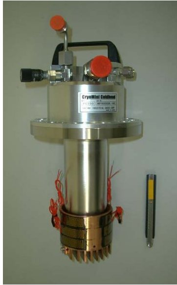
Figure 3.45: Pulse tube refrigerator for liquid xenon.
