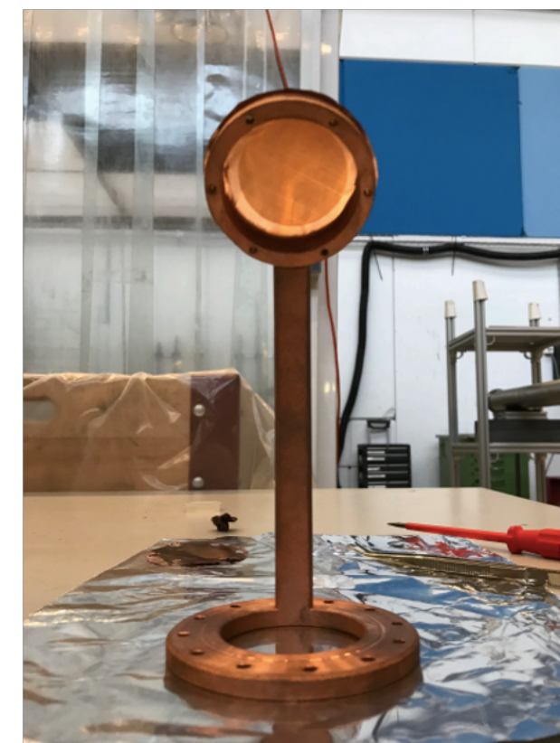
LiF target (INFN Legnaro) For BGO calibration
