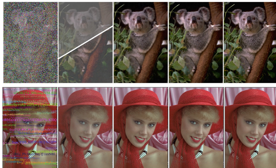
Input ( p \approx 0.25 ) 17.12 dB L_2 26.89 dB L_1 35.75 dB Clean targets 35.82 dB Ground truth PSNR
