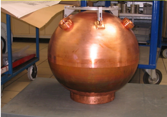
Low background detector d=60 cm p=10 bar
